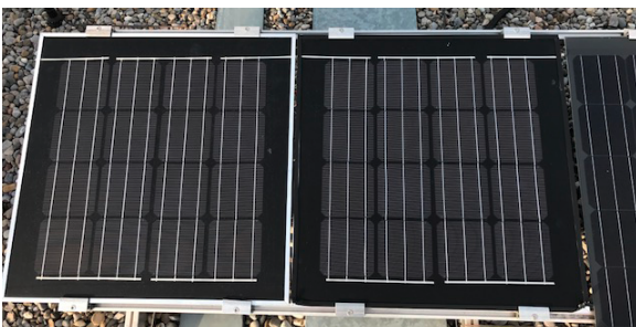
Fig. 4 Medium-area lightweight PV module composed of sixteen solar cells.
